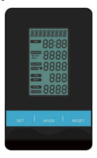
Display function of the console: TIME: User exercise time, setting range0:00-99:00(+-1:00) DIST (distance): User exercise distance, setting range 0-9990 (+-10)CAL (calories): User exercise calories, setting range 0-9990(+-10) SPM (speed): Display value according to the signal input.
